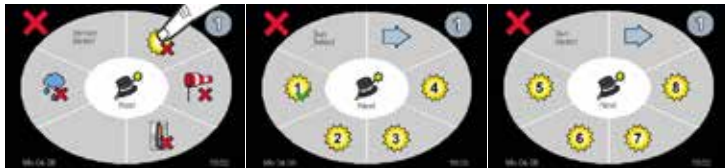
9. Selection of Lux sensor 10. Assignment of lux sensors (sun), sensors 1 to 4 11. Assignment of lux sensors (sun), sensors 5 to 8
