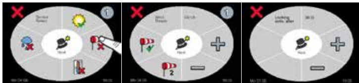
12. Selection of wind sensors 13. Assignment of wind sensors, setting wind limit and wind sensor 14. Setting wind sensor type: WM1 or WM2
